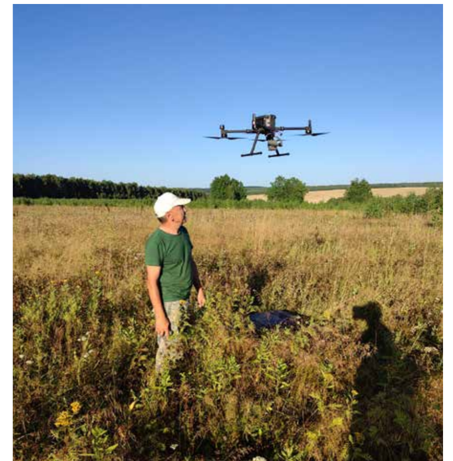
Departure of a Matrice 300 RTK drone with a lidar camera to scan a section of a carbon landfill
