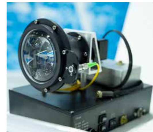
Laser gas analyzer for remote detection of methane emissions in UAV
